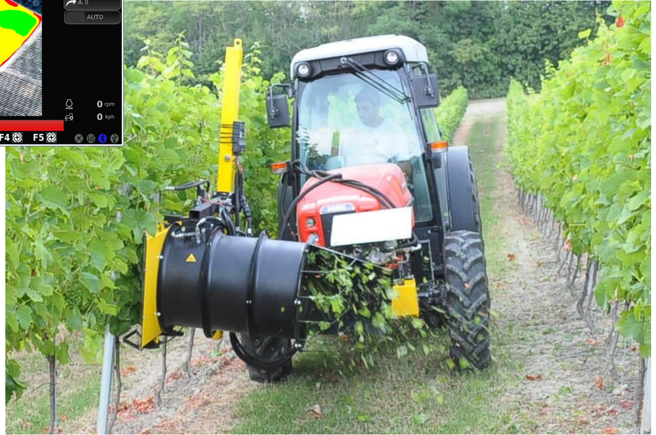
Vineyard leaf stripper with automatic tracking against canopy
